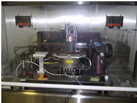
Figure 1. Scanning Kelvin probe with versatile gas systems
